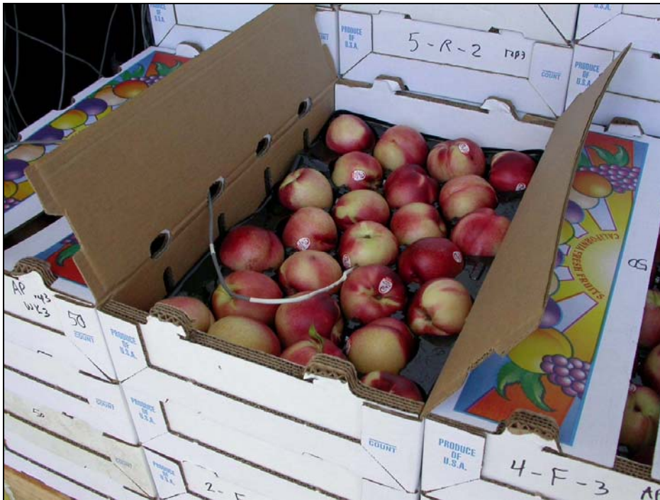
Figure 3. Single-layer box in chamber with temperature probe.
