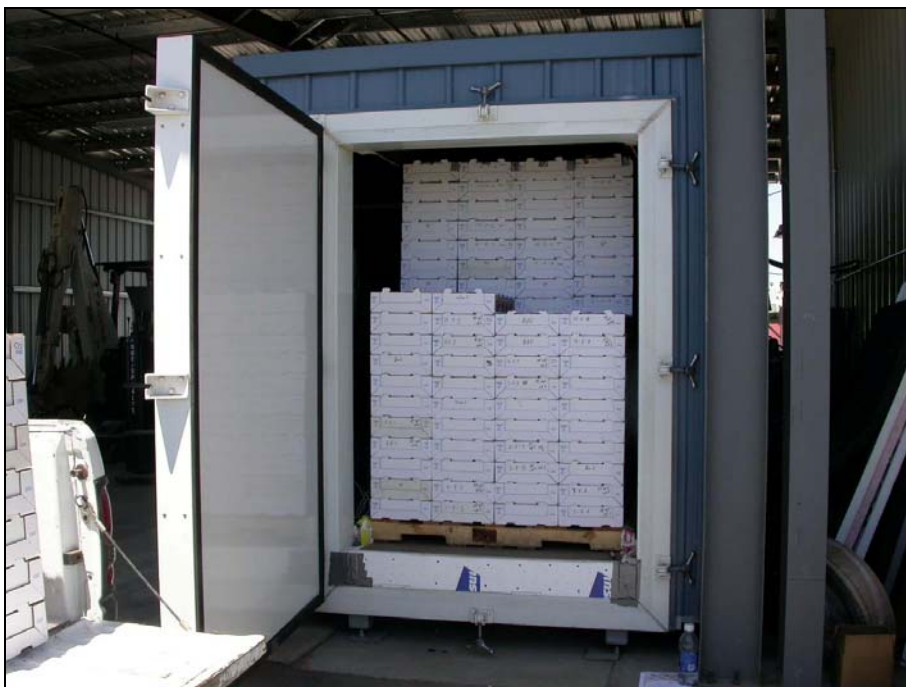
Figure 2. Picture of CATTS chamber partially-loaded with single-layer boxes
