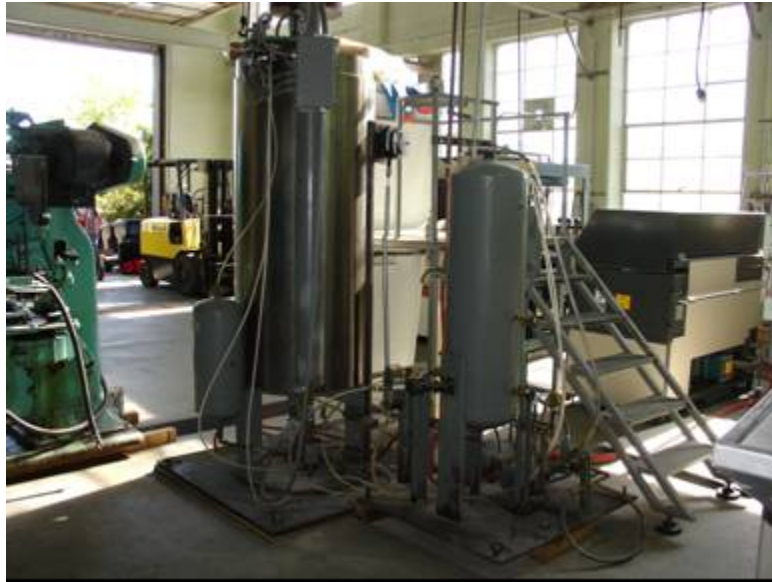
Fig. 1. Twenty-two liter high hydrostatic pressure vessel.
