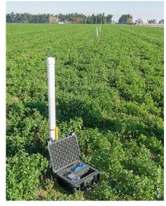
When a sensor (white pole) detects water arrival, a wireless signal is sent to the central module (black box), which generates a text message alert to the irrigator.
