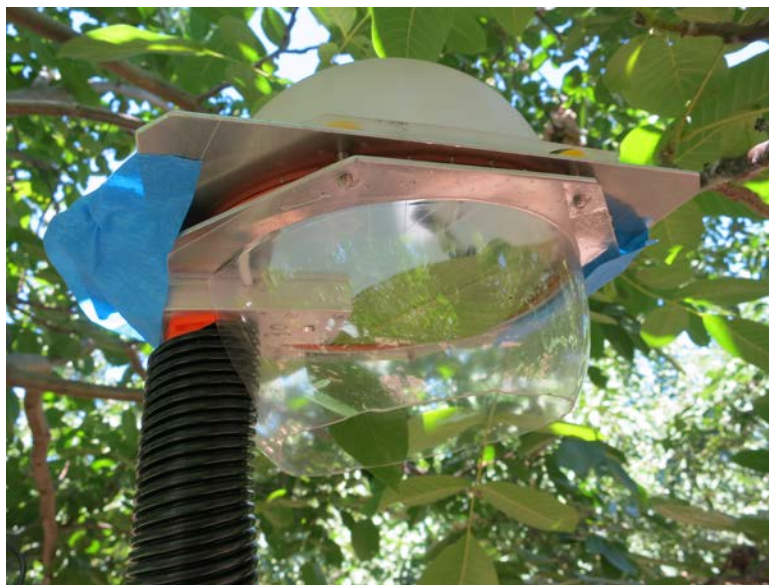
Figure 13: Leaf monitor installed in the lower, shaded canopy of a walnut tree.
