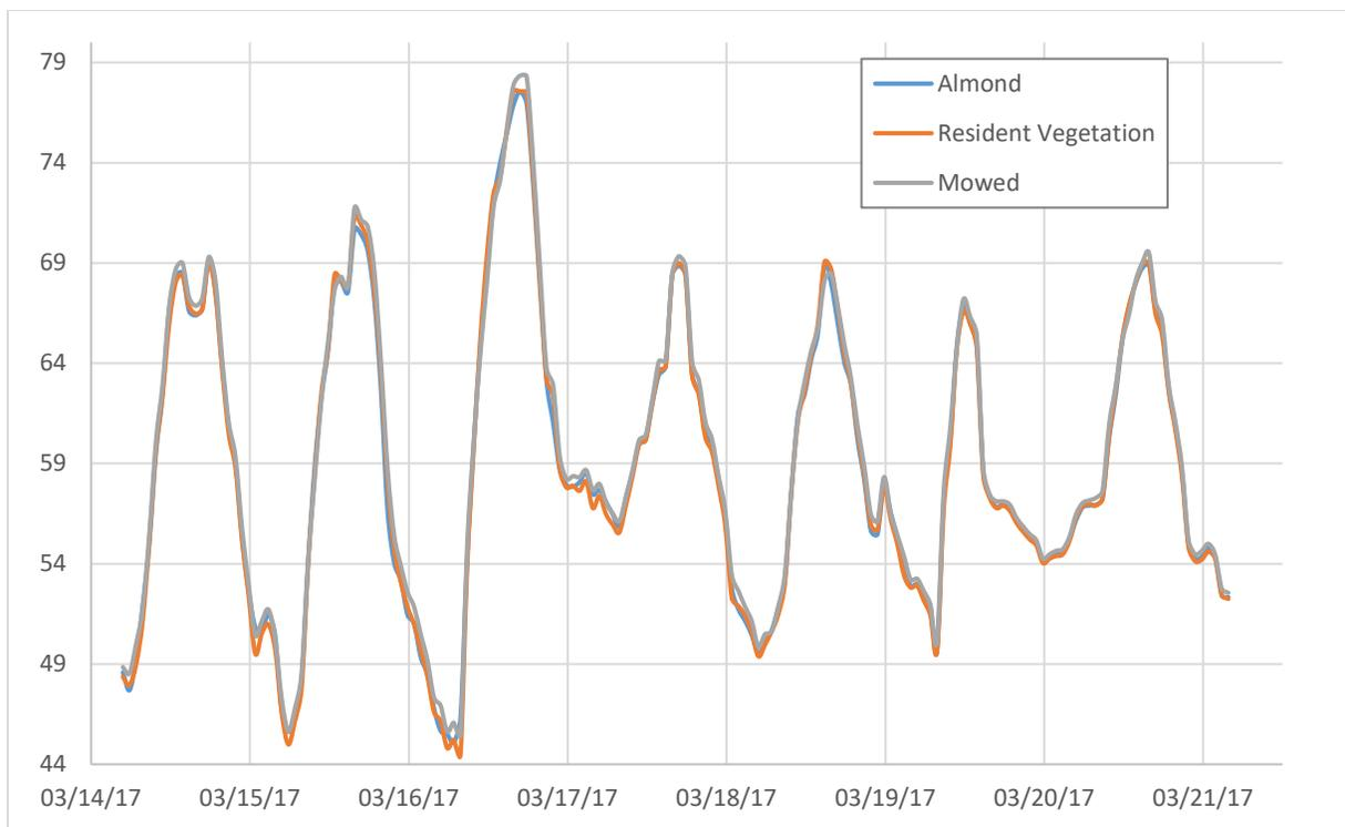
Figure 1. Temperature trace at the Orland site measured at 5 ft height in the tree row. Mowed vegetation was approximately 3 in. tall; resident vegetation was approximately 16 in. tall, and the cover crop in the adjacent almonds was approximately 5.5 ft tall.
