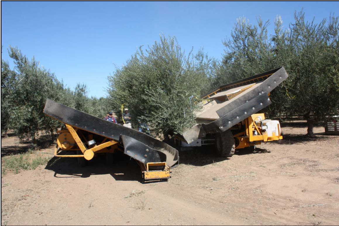
Fig. 2.1. ENE Inc. Terry II modified pistachio trunk shaking harvester with catch frame harvesting at Nickels Soils Laboratory on 5 October 2009. Mr. Terry Tompkins is operating the harvester.
