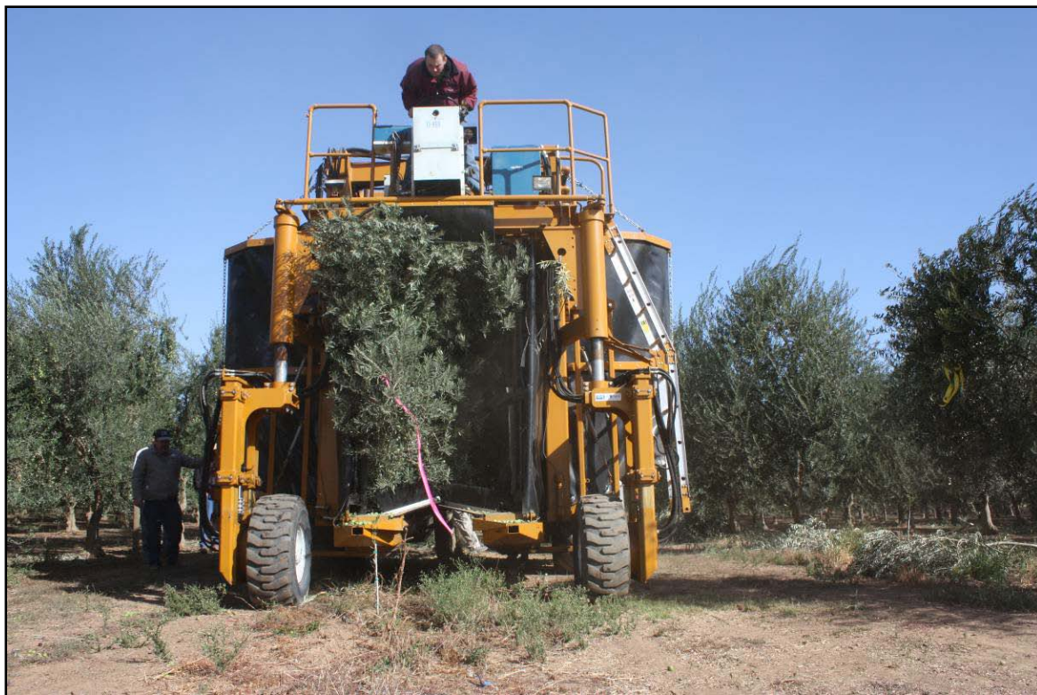
Fig. 2,2. Agright Olivia canopy contact head harvester operating in Nickels Soils Laboratory hedgerow olive orchard on 30 September 2009. Mr. Richard Loquaci of Madera Ag Services is operating the harvester.
