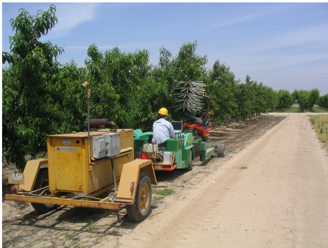
Fig. 1. Research apparatus assembled to evaluate the spiked-drum canopy shaker for using in the thinning of stone fruits at UC Kearney Experiment Station, (a: linear electric servo-motor, b: spiked-drum unit, c: UCD restored loader, d: electric and electronic power systems, e: 10kW three-phase generator).
