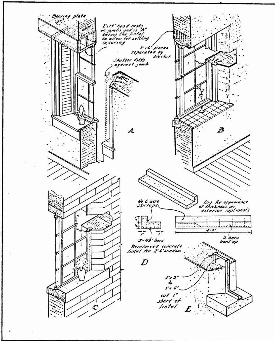
TYPICAL WINDOW DETAILS: A, Double-hung window, with standard sash adapted to splayed plank frame. B, Out-swinging wood casement, rabbeted 2 x 6-inch jamb, laminated lintel, "bull-nosed" plaster jamb, tile window ledge, brick sill, and roll screen. C, Steel casement window set in precast, reinforced concrete lintel. D, Reinforcing details for a precast concrete lintel. E, Steel sash on wooden T-shaped buck set in place in monolithic walls.
