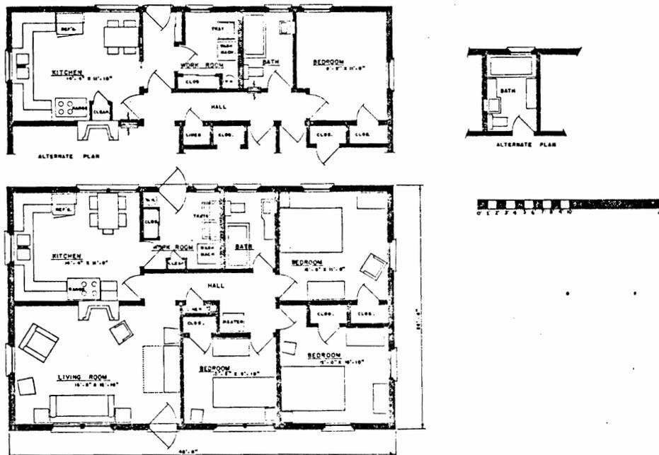
Three-bedroom house, 1,140 square feet. Principal dimensions are multiples of the 4-inch and 8-inch module, for economy and rapid construction. U-shaped kitchen provides storage and work space. A comfortable dinner area is near a large window. In alternate plan, the hall allows entrance from the rear into any room without going through work-room or kitchen.
