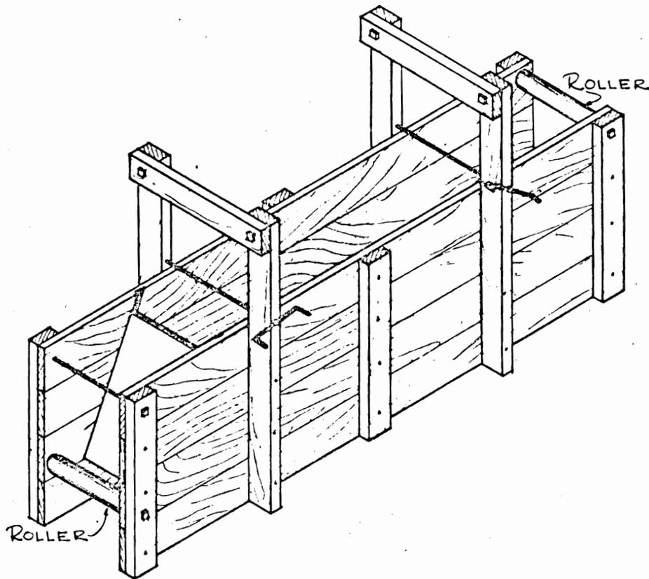
EASILY-MOVED ROLLING FORM built of  $1\frac{1}{4}$ " side boards, fastened to  $2" \times 4"$  studs and cantilevers. After ramming one section of wall, the form is moved to a new position by means of the two 3"-rollers. It does not have to be lifted. The form is held in place above the finished part of the wall by clamping it firmly with the two double-ended cranks.
