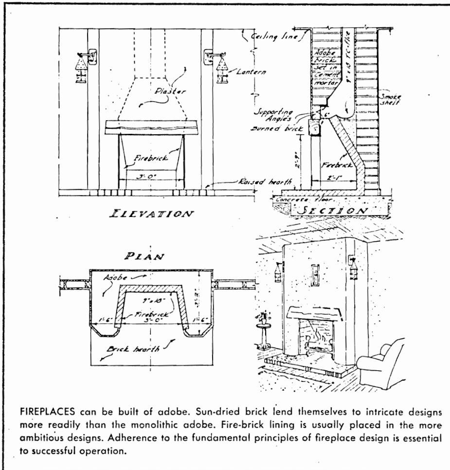
FIREPLACES can be built of adobe. Sun-dried brick lend themselves to intricate designs more readily than the monolithic adobe. Fire-brick lining is usually placed in the more ambitious designs. Adherence to the fundamental principles of fireplace design is essential to successful operation.
