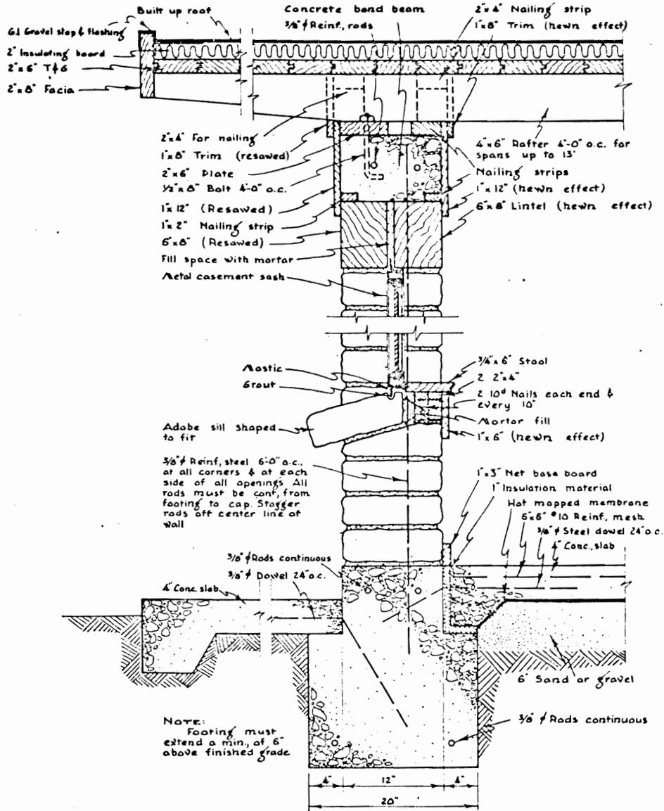
CROSS-SECTION DETAILS of roof, wall, floor, and foundation for typical adobe construction.
