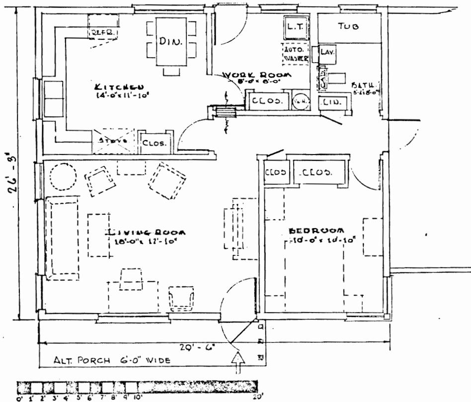
Plan for a one-bedroom adobe house, with a floor space of 774 square feet. Small, compact, can be expanded to three bedrooms. Roof may be gabled, flat, or shed type. Doors are placed so traffic does not cross work or living areas. Window location allows space for good arrangement of furniture and equipment.
