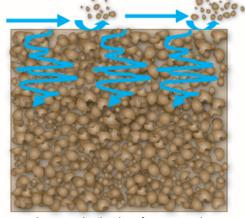
Compacted soil with surface crust and unstable aggregates
