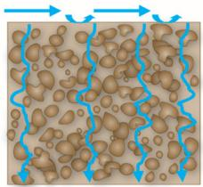
Uncompacted soil with stable aggregates
