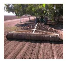
Figure 3. Spring tooth harrow breaking up the soil surface in an orchard. *Photo:* Terry L. Prichard
