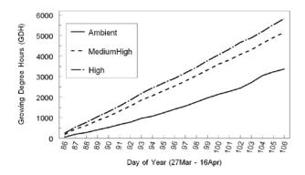
Figure 6. Accumulated heat units over the course of the experiments for ambient and the two temperature treatments.
