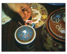
UC's 20-minute lead test uses citric acid to determine the presence of leachable lead in pottery.
