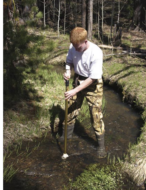
The researchers collected data in watersheds feeding Goose Lake, above ; the outlets of Lassen and Willow creeks are located on the peninsula in the center. Right , Shannon Cler, UC Davis postgraduate researcher, uses a velocity meter to estimate stream flow.
