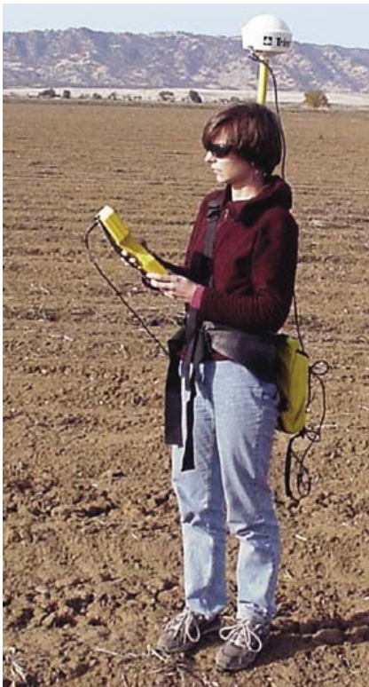
Left , former UC Davis graduate student Martina Koller uses a portable digital global positioning system (DGPS) and data logger to georeference samples and map weed population densities. Right , in the foreground, weed seedlings are light-green on the soil; in the background, the half-rate herbicide plots appear to be weed-free.
