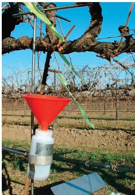
Stands were used to collect fungal spores disseminated in rainstorms. Left , each stand had a funnel under the cordon for estimating available inoculum within the vine, and a plate on the ground (2.5 inches high by 20 inches wide) at a 45° angle to collect splash from debris; right , stands also had two tented plates (8 inches high by 12 inches wide), which were designed to collect wind-blown rain.
