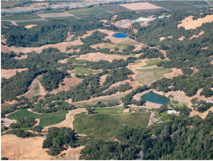
Aerial photography of vineyards, coupled with stream-flow data, is being used to develop models that will help growers and regulators to better plan for future water needs and salmon recovery. In, left, Alexander Valley and, right, Dry Creek, vineyards grow on hillsides.
