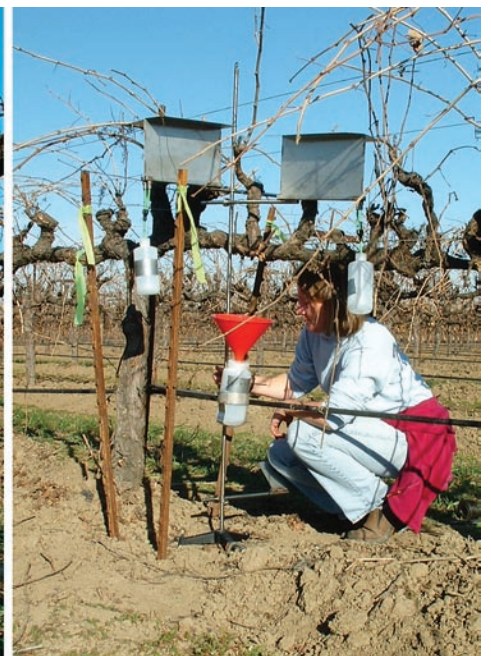
Stands were used to collect fungal spores disseminated in rainstorms. Left , each stand had a funnel under the cordon for estimating available inoculum within the vine, and a plate on the ground (2.5 inches high by 20 inches wide) at a 45° angle to collect splash from debris; right , stands also had two tented plates (8 inches high by 12 inches wide), which were designed to collect wind-blown rain.
