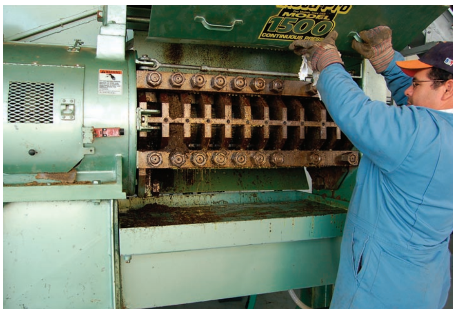
German Perez uses a press to extract oil from mustard and canola seeds, which were irrigated with water high in salt, boron and selenium. Under experimental conditions, the press can process up to a ton of canola seed per hour with an oil-extraction efficiency of nearly 90%.
