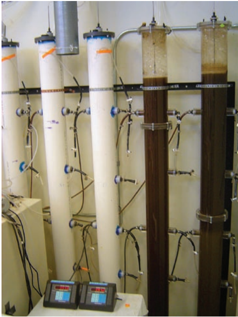
Laboratory-scale reactors were used to test the effectiveness of various manure treatments.
