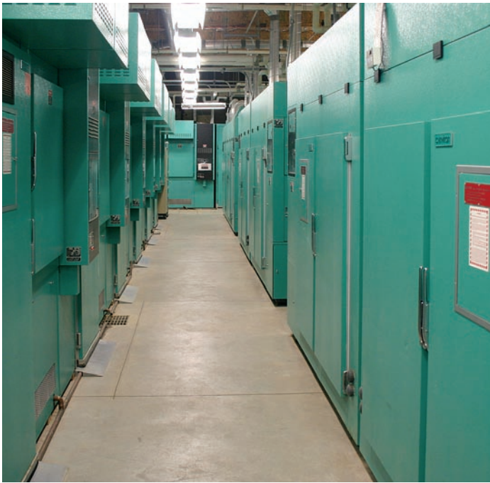
Environmental chambers in the UC Davis Controlled Environment Facility are helping scientists to understand how plants react to changes in atmospheric carbon, oxygen and other greenhouse gases.
