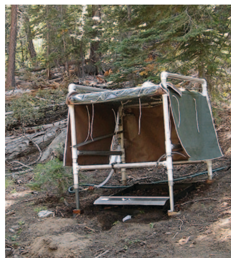
A rainfall simulator, above, at Bliss State Park was used at different rates to generate runoff and measure its sediment content.
