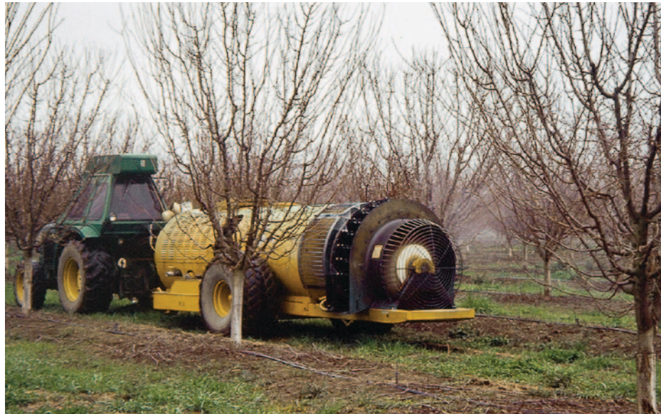
A commercial sprayer retrofitted with a target-sensing spray system applies dormant spray in a prune orchard near Chico. These "smart" systems only apply sprays where a tree is detected.
