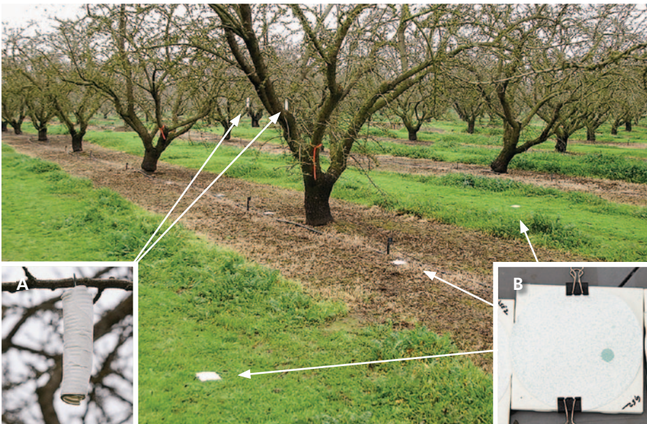
To monitor the tree and ground deposition of spray applications, (A) 1-inch-diameter cylinders fitted with fiber filters were suspended from almond trees at different heights and (B) 4.25-inch glass filters supported by flat ceramic tiles were laid on the orchard floor.
