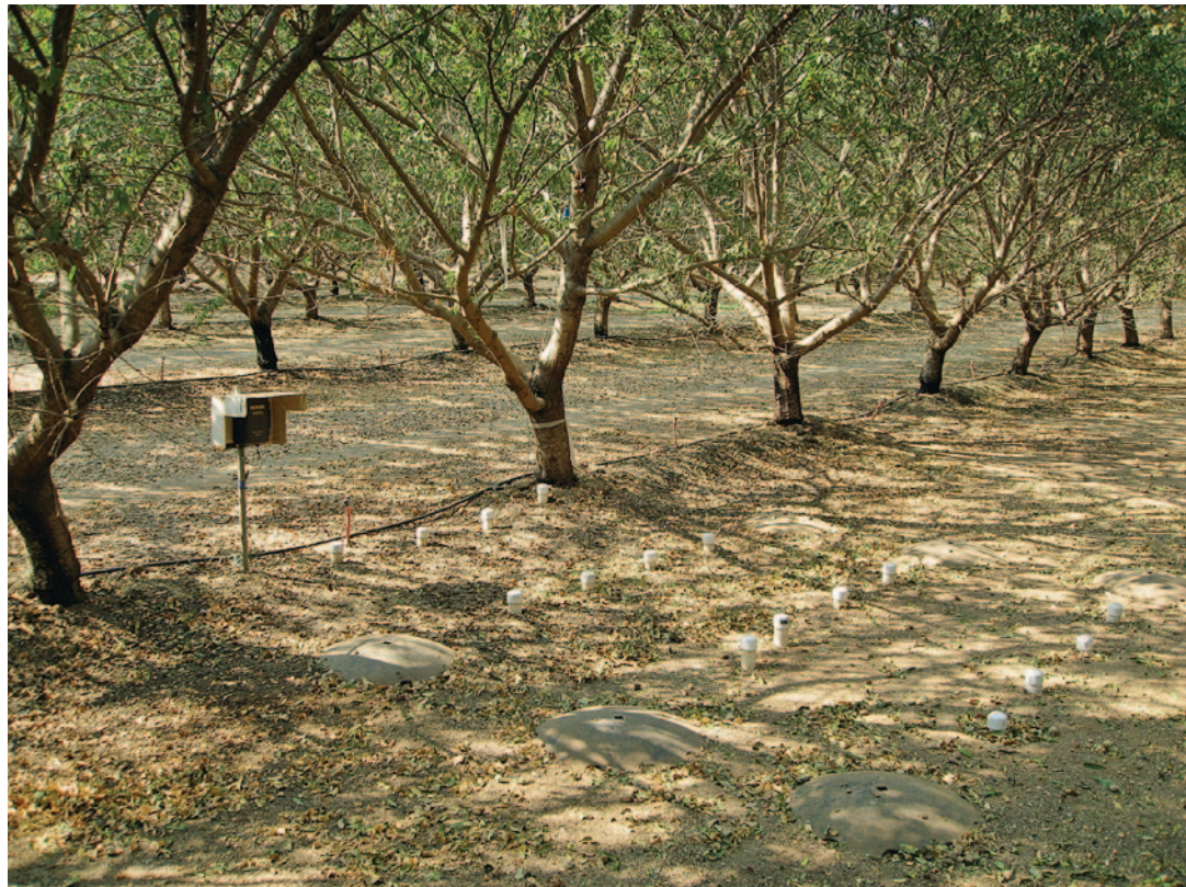
Grids of neutron-probe access tubes allowed the researchers to take soil moisture readings at different depths. They found a shallow water table that receded throughout the growing season, especially during two drought years.
