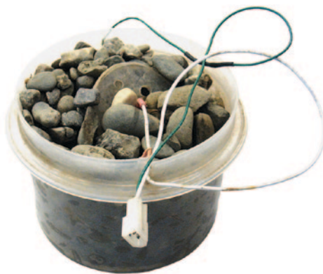
The wetting-front sensor consists of a plastic container surrounded by a gravel and sand jacket.
