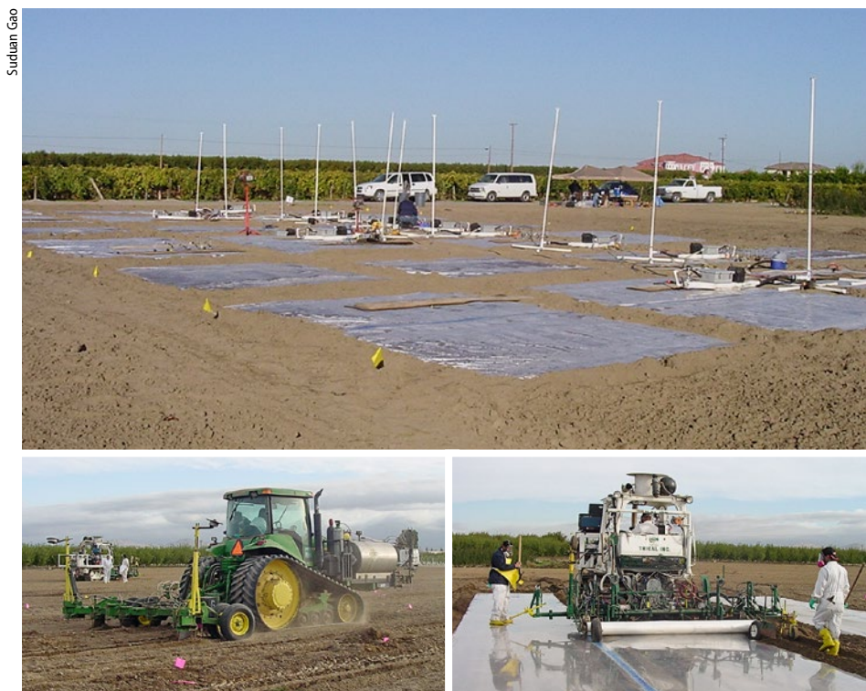
Researchers used dynamic flux chamber equipment, top , to measure fumigant emissions throughout the fall 2009 trial period and 24 hours after tarp cutting. Bottom left , fumigant injection; bottom right , plastic tarp installment at Parlier, Fresno County.
