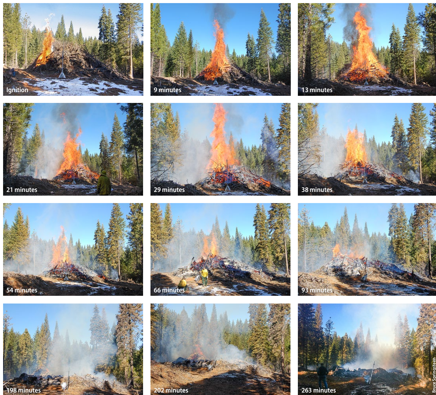
Fig. 3. In 2014, researchers measured air emissions from an open pile burn at BFRS. Due to the size and height of the burn, they were unable to sample the main section of the plume during the full flaming combustion mode (see time interval at 13 minutes). Flaming phase transitioned to smoldering phase approximately 40 minutes after ignition.
