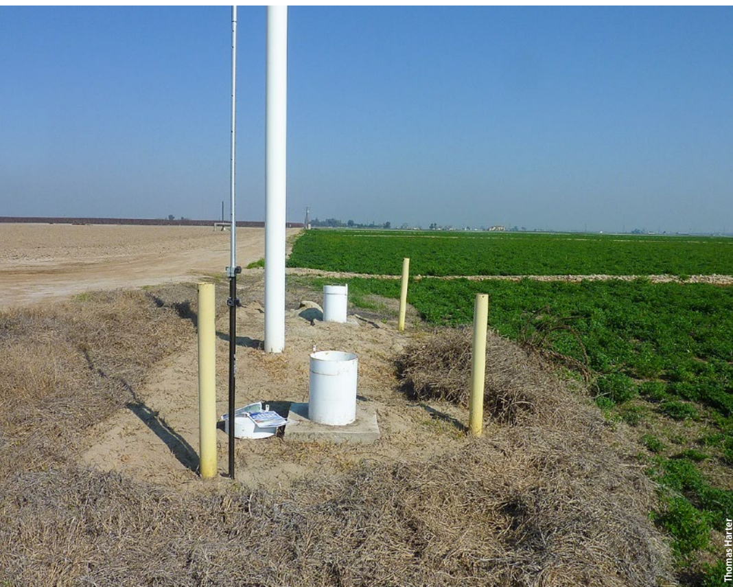
Two monitoring wells (short white casings) adjacent to an irrigated, manure-treated field as part of a dairy monitoring program.
