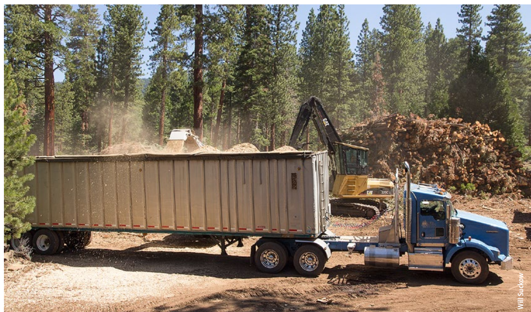
A trailer is loaded with wood chips at a U.S. Forest Service-funded fuels reduction project in the Lake Tahoe area. The chips will be hauled to a biomass energy facility to help defray disposal costs.
