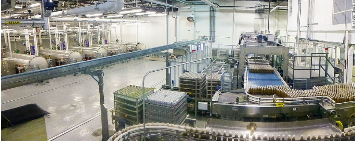
This beverage unit installed by AgPLUS partner JBT FoodTech can process up to 600 containers per minute.
