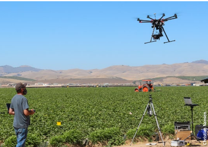
Robert Starnes, a senior superintendent of agriculture in the UC Davis Department of Entomology, flies a drone over a field of strawberries in San Luis Obispo County to study how reflectance data may help detect outbreaks of spider mite, a common pest.
