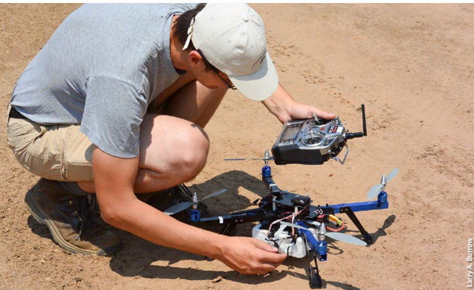
Andreas Anderson, an instructor with the Center for Information Technology Research in the Interest of Society at UC Merced, checks the control systems for a drone-mounted multispectral camera before a research flight in Merced County for a study on water stress in almond trees.
