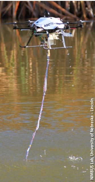
A drone-mounted thermal sensor can monitor temperature in a water body or watercourse at various depths and times of day, helping to identify habitat zones for aquatic species.
