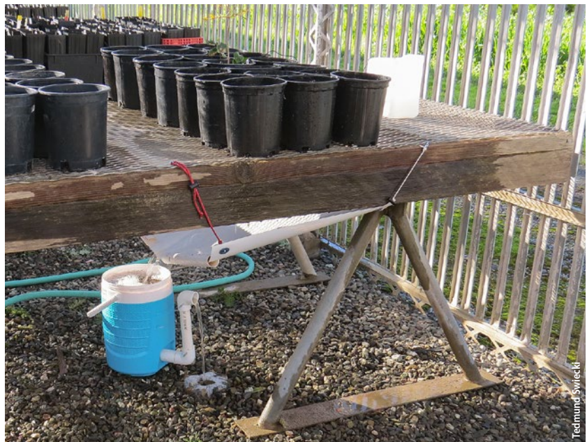
Leachate collection systems and zoospore collection vessels under arrays of 42, top , and 21, bottom , #1 container plants. Each array contains one known Phytophthora -infected plant. Remaining pots are filled with pasteurized potting media (seeded with turfgrass, top ).
