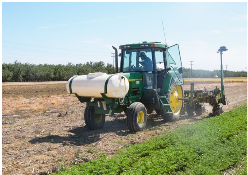
No-till sorghum seeding on May 22, 2017, into an NTNO (no-till, no cover crop) plot using a 6-row John Deere 1730 no-till seeder. On the lower right, there is an NTNO garbanzo plot. Photo: Jeffrey P. Mitchell.
