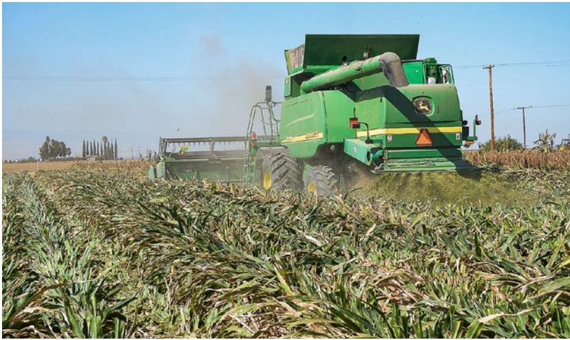
Thirty-foot wide combine harvester used for sorghum grain and garbanzo harvests. Photo: Jeffrey P. Mitchell.
