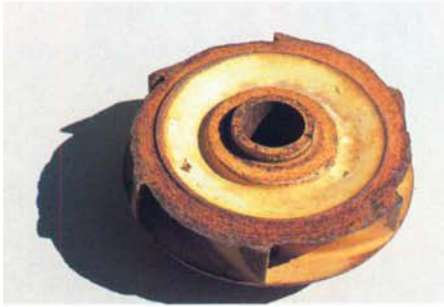
Worn impeller and a centrifugal pump.
