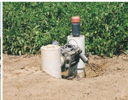
Left, A set of filters prevents irrigation water from clogging the drip lines. Right, Pressure-regulating valves allow growers to control the pressure of the irrigation water flowing into the drip line.
