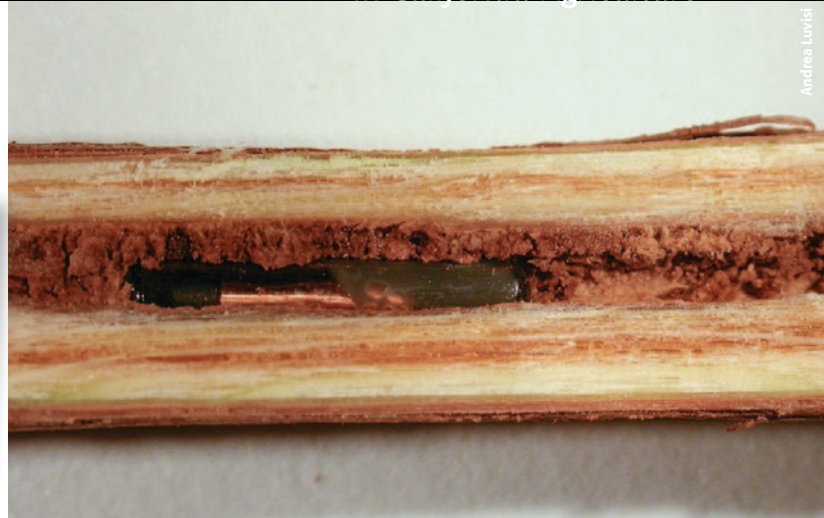
Longitudinal section of grapevine with implanted RFID microchip
