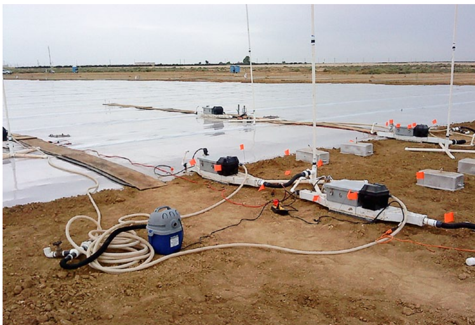
To monitor fumigant emissions at ground level, researchers used dynamic flux chamber equipment, above, to confirm and interpret the ambient air monitoring data.
