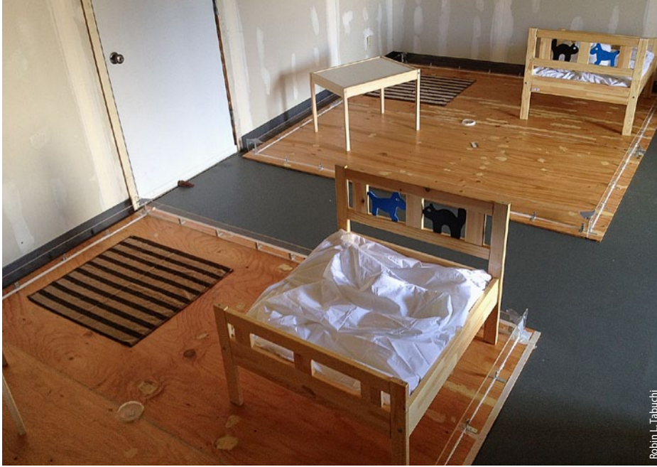
Layout of wooden testing arenas inside the Villa Termiti at UC Berkeley's Richmond Field Station used for simulated field tests of the performance of active and passive bed bug monitors.
