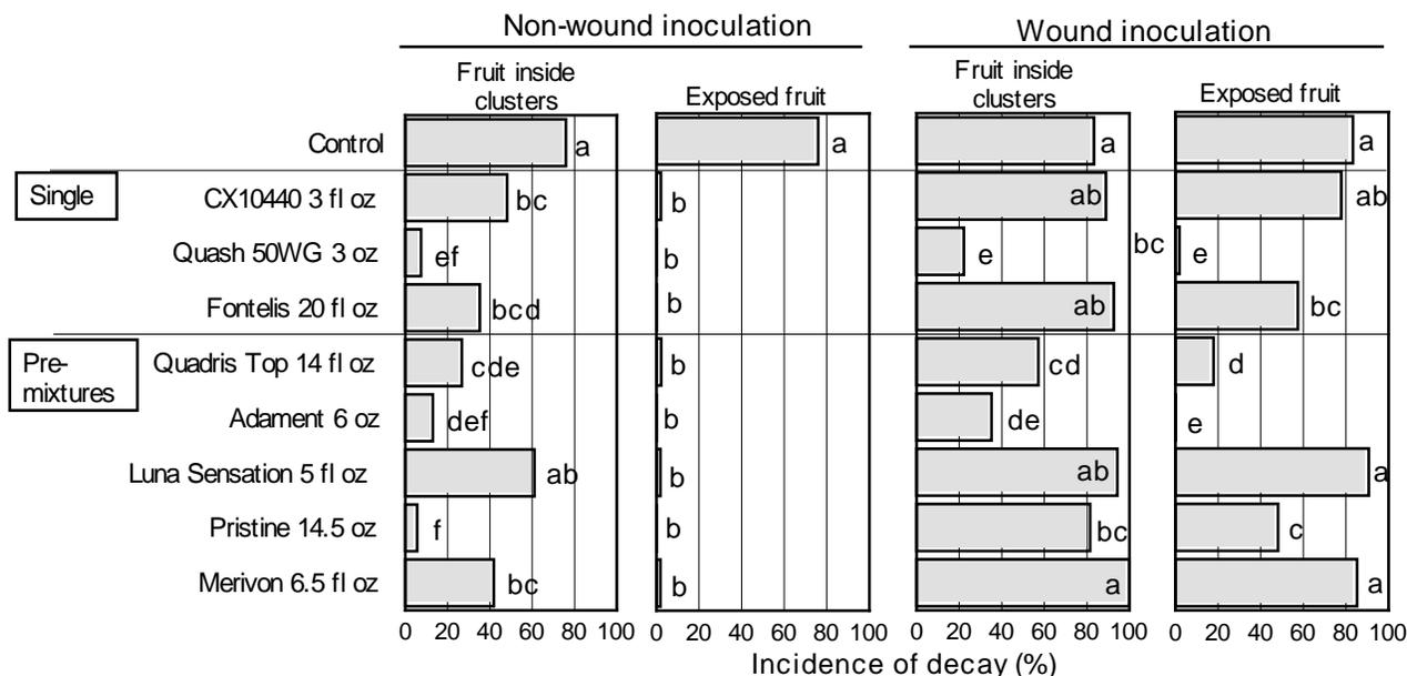
Treatments were applied in the field on 8-16-12 in combination with Omni Supreme Spray Oil (1.5%) using an air-blast sprayer at 130 gal/A. At harvest, fruit from the tree perimeter (exposed fruit) and from clusters were collected and wound- or non-wound-inoculated with conidia of *M. fructicola* (30,000 conidia/ml). Fruit were then incubated for 7 days at 20 C.
