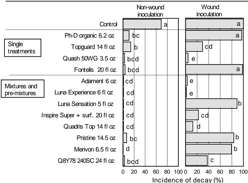
Treatments were applied in the field in combination with Omni Supreme Spray Oil (1.5%) on 8-16-12 using an air-blast sprayer at 130 gal/A. After harvest, fruit were non-wound- or wound-inoculated with conidia of *M. fructicola* (30,000 conidia/ml) and then incubated for 7 days at 20 C.
