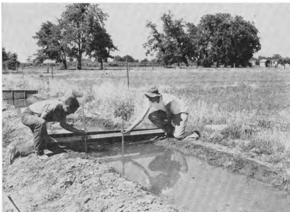
Making measurements during a seepage ponding test.
