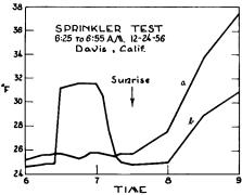
Temperature rise during sprinkling—curve a. As operation was stopped before sunrise the sprinkled bulb cooled to previous temperature and stayed colder than the outside control bulb —curve b—until the ice crust had melted and the water had evaporated.
