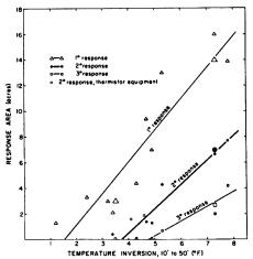
Plot of 12 test runs in the Chico almond orchard. The diagrams below are shown as bolder points. This graph plots the acreage within the isolines for the 1°F, 2°F, and 3°F responses against the inversion strength in °F. The straight lines are calculated lines of best fit, and provide a reasonable evaluation of wind machine performance under these conditions.
