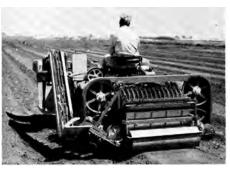
Cutting blade, conveyor, and roller of the second model asparagus harvester.
