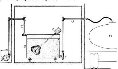
Diagrammatic illustration of tank truck picking up milk from a storage tank in the farm milk-house. A. Dump vat. B. I-inch milk pump. C. Surface cooler. D. Farm storage tank. E. Agitator. F. 1/2-inch milk pump. G. Sanitary pipe line. H. Insulated stainless steel tank on truck.
