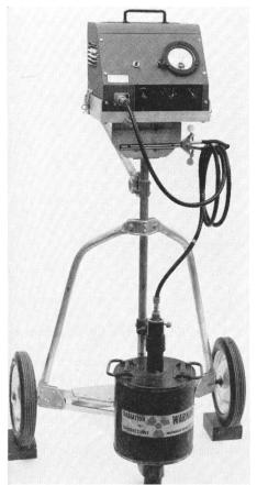
equipment, 36'' concrete drain tiles were used to contain soil columns from 30''to 42'' deep. An aluminum access tube was centrally located in each soil column. The tubes extended from  $21/_2''$  above the soil surface to the bottom of the column. The tubes provided mechanical support for the neutron equipment and an opening through which to lower a moisture probe into the soil.
