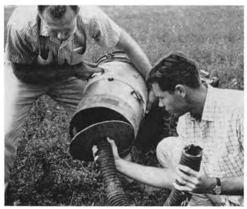
Placement of adapter hose for complete sampling.
