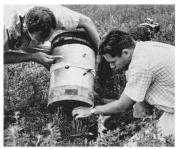
Clipped stems within nozzle shaken to loosen insects.
