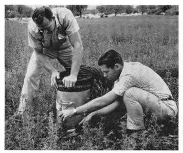
Cutting alfalfa encircling the nozzle of sampling machine.
