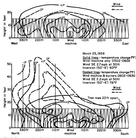
Vertical cross-section showing the temperature changes (°F) on March 25, 1959. Note the schematically presented trees and the solid heavy vertical lines which indicate the masts for the temperature sensing instruments.
