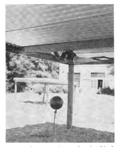
View under a test frame showing black globe thermometer used to measure radiant heat load and hemispherical radiometer to measure radiation received by underside of test material.
