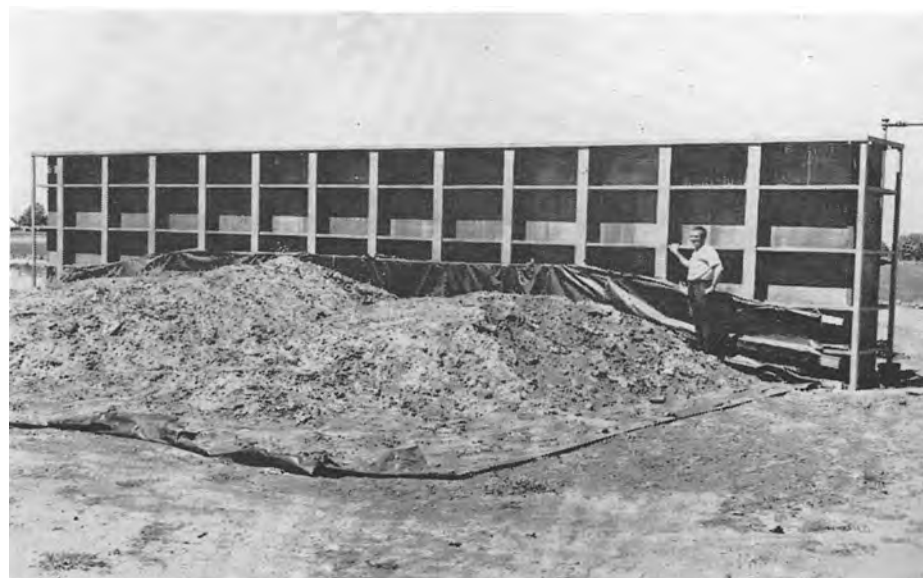
One of the tanks being used on the Davis Campus in making soil drainage tests. The soil in the foreground will be put into the tank.
