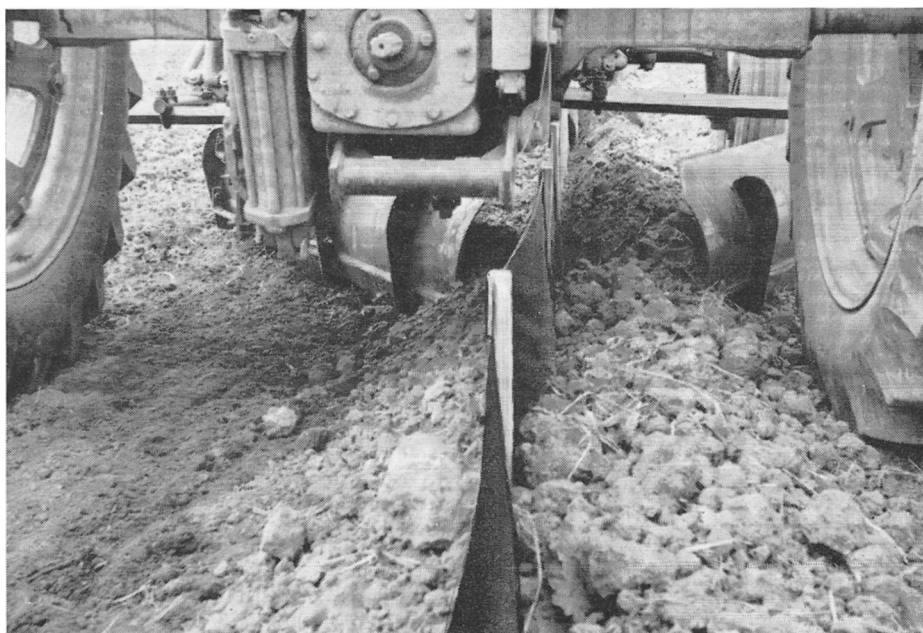
Backfilling furrows with plastic levees in place using V-blades under tractor.
