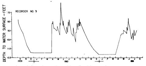
Fig. 4—Chart of hydrographic recorder No 9 located 1800 feet east of Pump No. 1.
