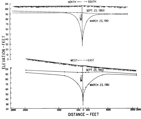
Fig. 2—Water table profile chart at Pump No. 1.
