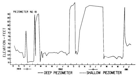
Fig. 3—Water table fluctuations in 80 foot piezometer located 50 feet east of Pump No. 1
