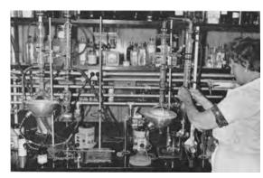
Use of this hydrolysis apparatus in the colorimetric analysis of herbicides, is one of many painstaking laboratory procedures conducted in departments at all campuses to produce scientifically exact information on the safe use of agricultural chemicals.
