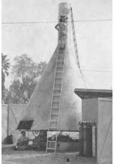
Burning tower and laboratory, to right, with technician checking scales as fuel is burned and another technician, on ladder, checking a velometer, mounted outside the upper stack, which records air flow as transmitted electronically from an anemometer mounted inside.
