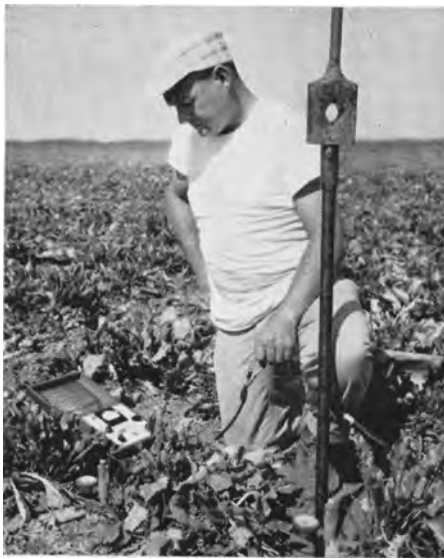
Tensiometers, electrical resistance blocks and soil samples were used by the Irrigation Department to determine soil moisture content in sugar beet test plots at Davis.
