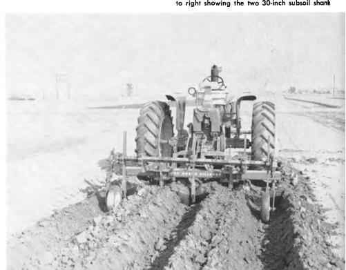
Beds with subsoil slot directly below intended drill row are seen in phy to right showing the two 30-inch subsoil shank
