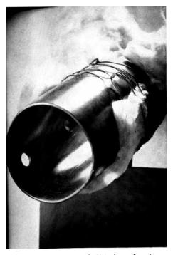
Four-inch plastic tile with %-inch perforations, wrapped with glass fiber envelope.
