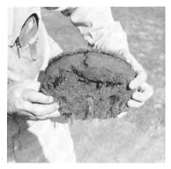
Section of turf shows good grass root growth through backfilled material in drilled holes in renovation test.
