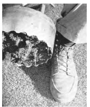
After removal of  $1\frac{1}{4}$  to  $1\frac{1}{2}$  inches of thatch and soil, the penetration rate was  $\frac{1}{4}$ -inch per hour. When 4 to 6 inches of the stratified, compacted material was removed, the parent soil was found to have a rate of infiltration of approximately 2 inches per hour.
