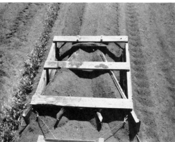
Bed shaper used on machine-cut rows, shown in peat field.
