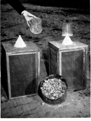
Poultry droppings were kept in metal containers inside screened enclosures seen in photo until all emerging adult flies were trapped in container at the top of the cage, and killed by exposure to an insecticide-impregnated strip of cloth.
